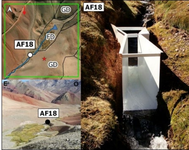
Figure 3. "Cutthroat flume" in the Chasquillar streamlet, at the lower section of the homonymous basin (see reference for detailed figure 3).
