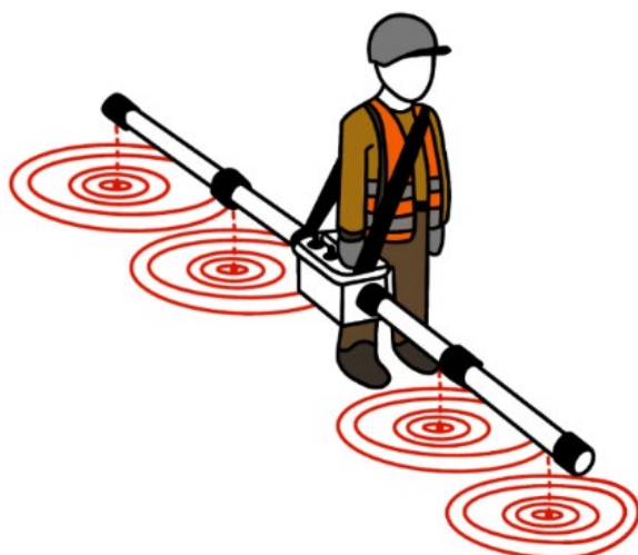
Figure 5. Diagrammatic sketch of EM-31 instrument assembled to conduct a field survey.
