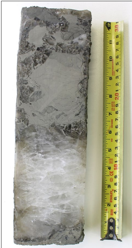
Figure 2. Ice-rich permafrost showing thick layered (top) and suspended (base) cryostructures in a core from BH1 at a depth of 657 cm.
