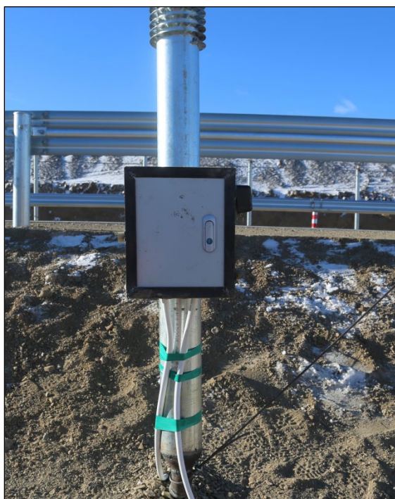
Figure 4. Monitoring box: temperature sensors are installed in white PVC tubes at the end of the evaporator tube and between the thermosyphons.
